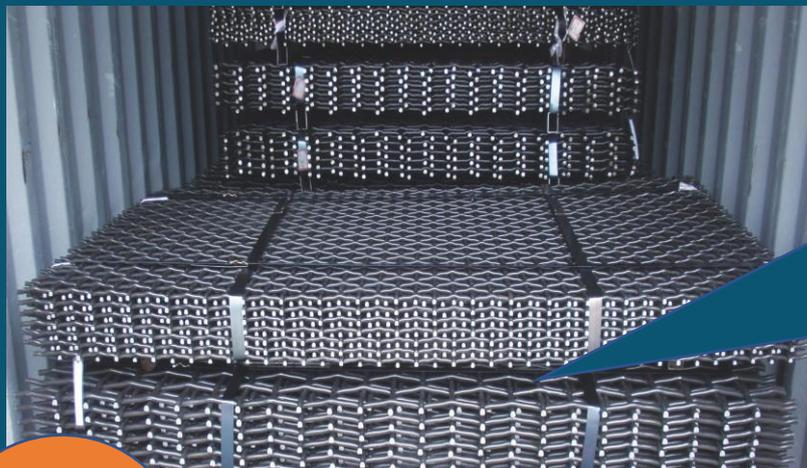
Wire spur should be cut neat. Spur Length should be longer than the wire diameter, but be shorter than half of an aperture. Though it is not a quality problem. But it will be troubles when installation.
