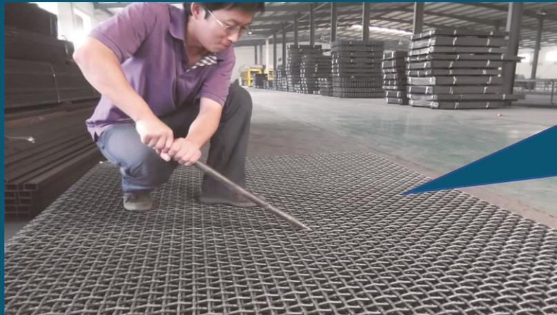
Good Quality woven mesh has zero tolerance to any movement within crimp or weave. Tight weave improves wear life in the field.
